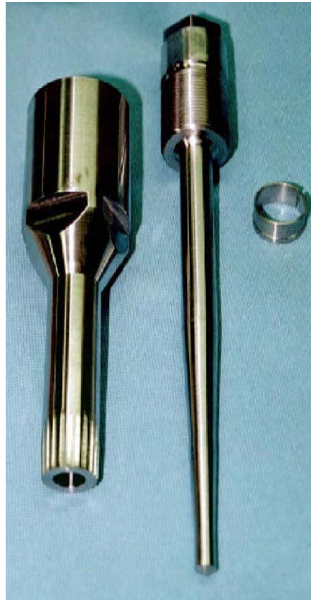
Fig. 3. Photograph of 3/4 thermowell nozzle design.
